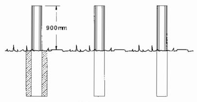
Bollards embedded approximately 750 mm and surrounded with 100 mm mass concrete
